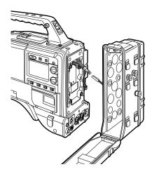
Mount the AU-M402H battery case.
